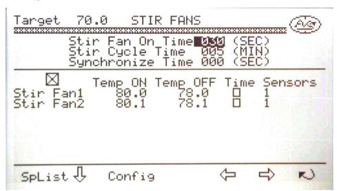
Target Target temperature according to Growth Day and Ramping. This value can not be changed on this screen.
