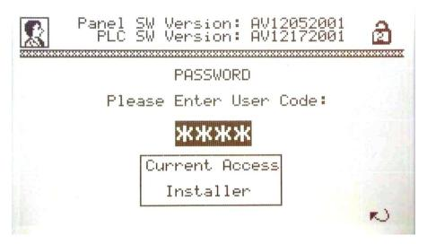
This screen enables the user to put in codes that will limit access to the output configuration, and the system settings.
